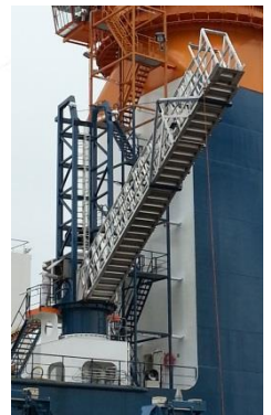
Extendable gangway with Tower-Crane.
